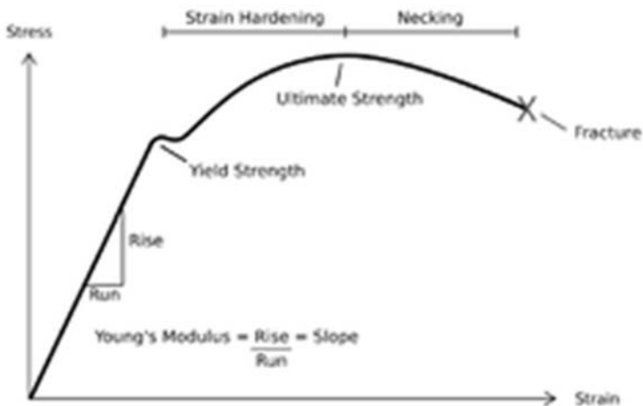
Figure 4. Stress-strain curve
