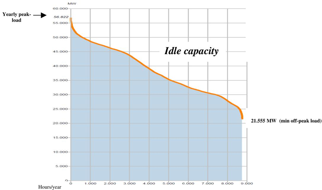
**Figure 2 – Italy’s yearly (2007) load duration curve.**
