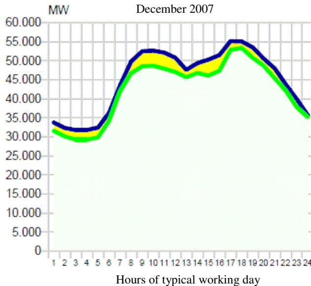
The higher curve represents the hourly power demand, while the lower curve represents the corresponding power produced in Italy. Their difference is equal to the power imported from abroad.
