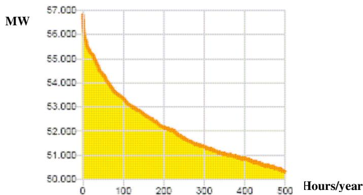
**Figure 3 – Zoom of the load yearly duration curve of the 500 hours of peak-load**
