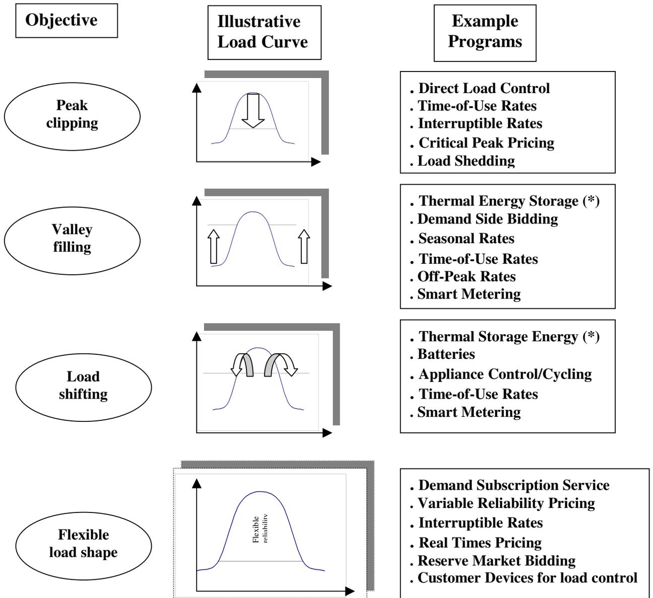
**Figure 8 – Load management load shape objectives**
