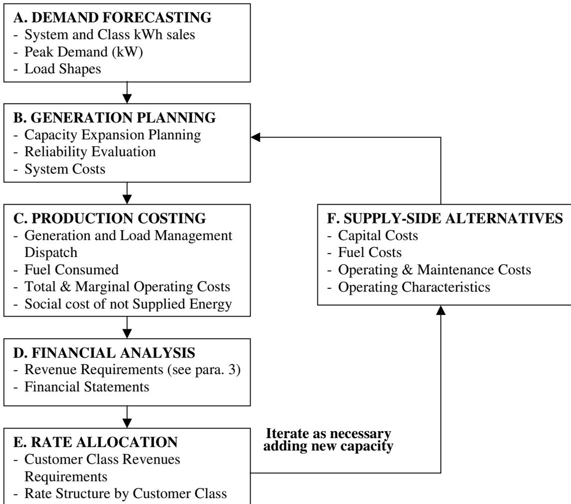
**Figure 4 – Supply Side Planning Process**
