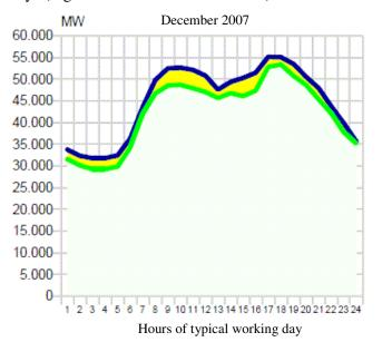
The higher curve represents the hourly power demand, while the lower curve represents the corresponding power produced in Italy. Their difference is equal to the power imported from abroad.
